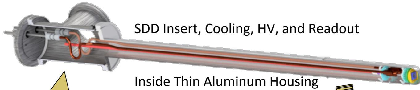
SDD Insert, Cooling, HV, and Readout
